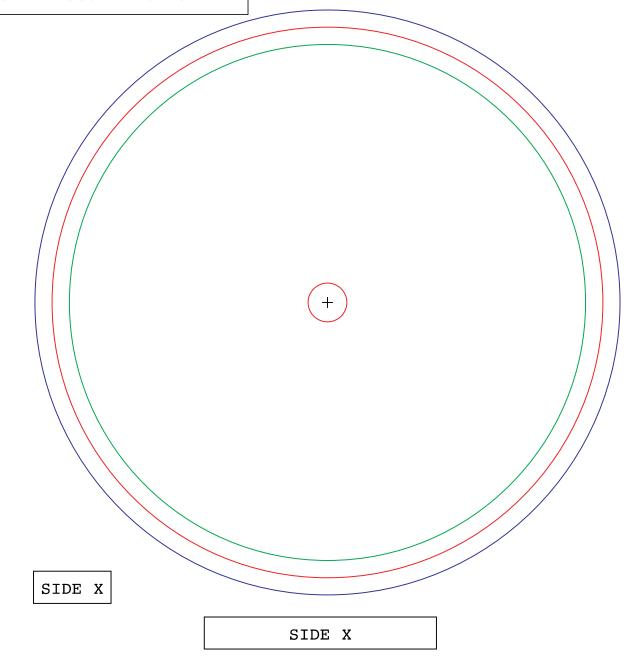
Outer Diameter cut:101.6 mm Inner Diameter cut:7.14 mm
